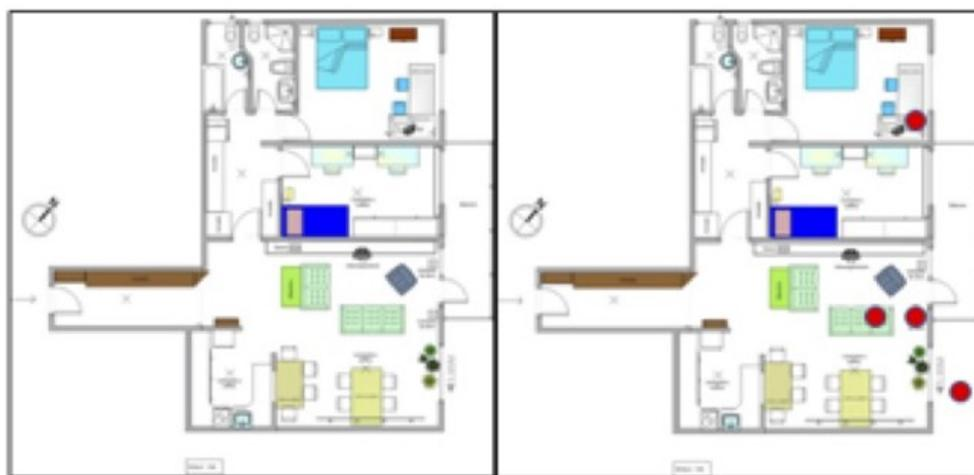
Figure 1: Home-mapping for tracking activities, based on the home map (left side). The movements of the family members are indicated over time within the spaces they occupy (the red elements on the right side) [14]
